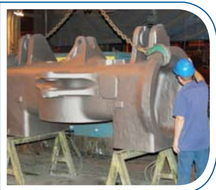
Large mining truck differential
